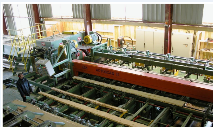
3D Scanner Optimizer for Boards and Cants with automatic infeed table for optimal recovery and high productivity.
