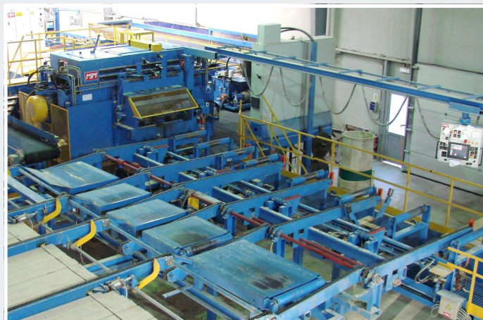
Manual infeed table with idle rollers, centering system, pneumatic turner for boards and cants.
